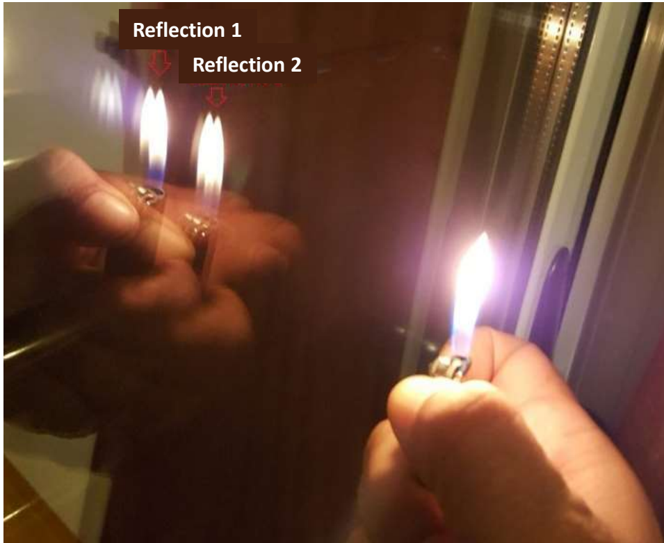
Check of Low-e energy-efficient glass
